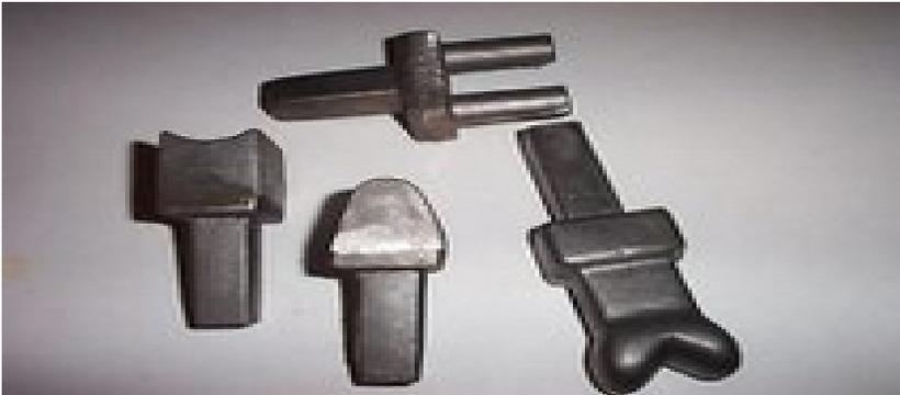
Fullers: Similar to swage. Top has a wooden handle and bottom has a plug for the hardie hole. Used in pairs.
