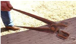
Round bit tongs: Curved bit. Used for holding round iron.
