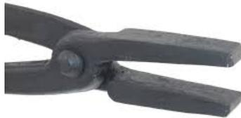
Box tongs: For holding square iron. Has a lip on the inside to keep the iron from slipping out.
