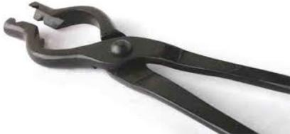
Hollow bit tongs: Has a hollow area at the end to hold a round piece with a swell (Such as a bolt).
