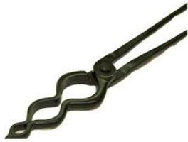
Flat tongs: Bit is flattened to hold flat pieces of iron.
